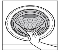
Check the folds of the door seal for any small articles which may have been trapped.
